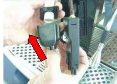
**4** ▶ Disassemble the milk frother in all its parts (first by turning and then by pulling as shown in the picture) and wash it either by hand or in a dishwasher. Make sure that all the holes are free from milk residues and also to use provided tools to clean the holes. Check also that the O-rings are in good condition
