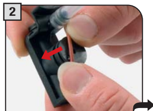
Insert the new O-ring pressing it delicately.
